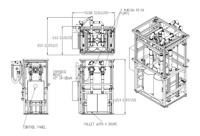
The Murzan ABDT juice concentrate unloading system consist of two double diaphragm pumps that are mounted on a stainless steel carriage that moves the pumps and suction wand up and down to allow entrance and unloading of the four drums on a pallet at the same time.
